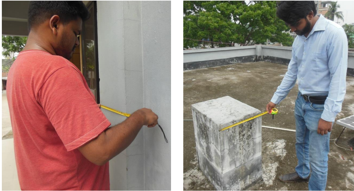
Figure 6.3: Measuring of physical dimension of column
