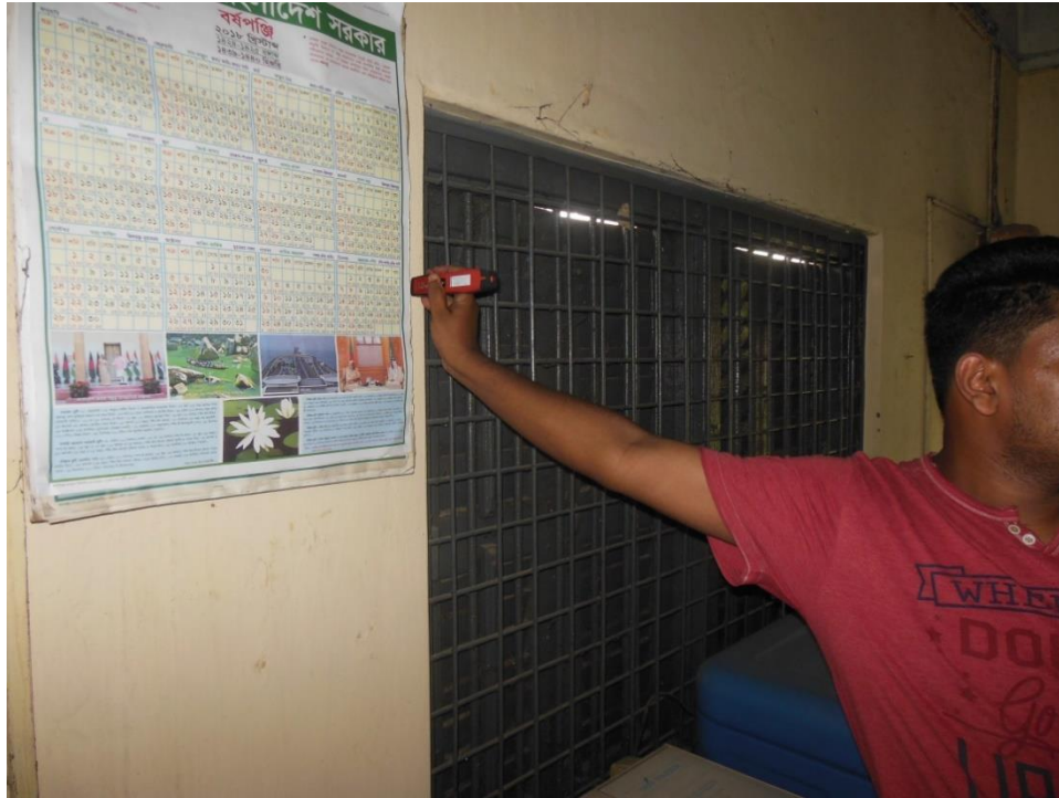
Figure 6.6: Measuring physical dimension of the building using laser meter
